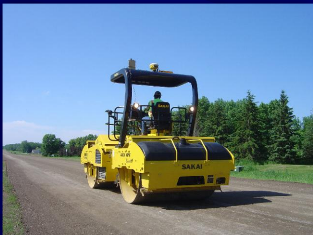
Sakai double-drum IC roller
