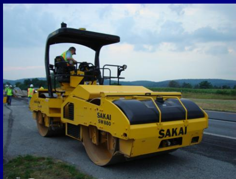
Sakai double-drum IC roller
