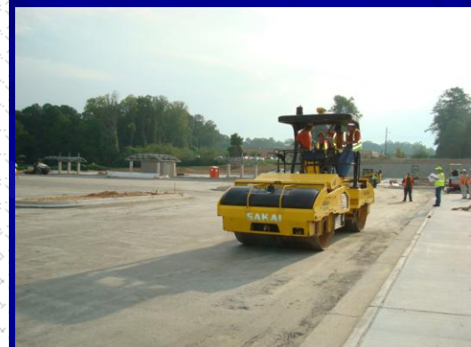
Sakai Double-drum IC roller
