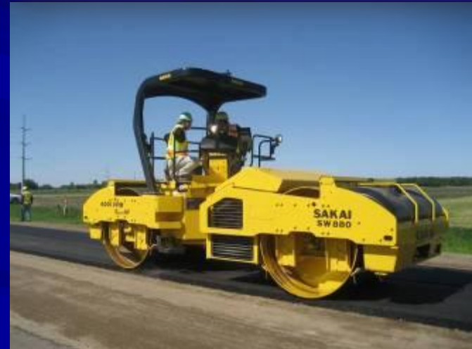
Sakai double-drum IC roller
